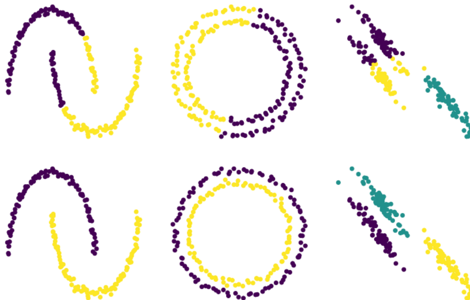
Figure 1. Results of clustering on dummy datasets. The first row shows the results of k-means clustering, while the second row shows the results of spectral clustering.
