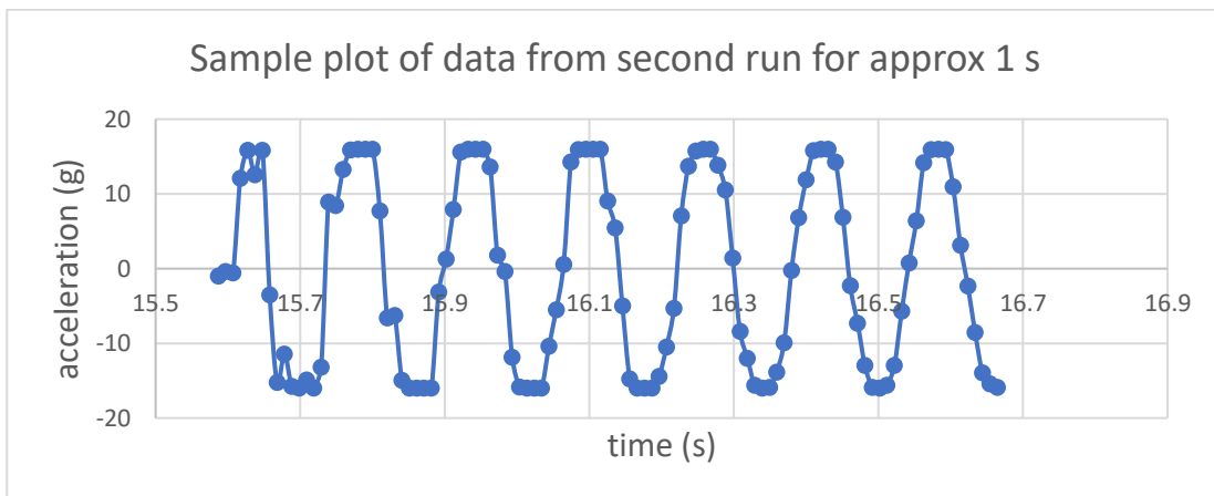
Figure 5: Vertical acceleration of the shaft tip in the second run after the load is removed
